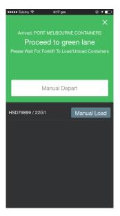
As the forklift operator loads the container onto your vehicle, the information they enter into their Forklift Mounted Terminal (FMT) will update the information in the driver app.
